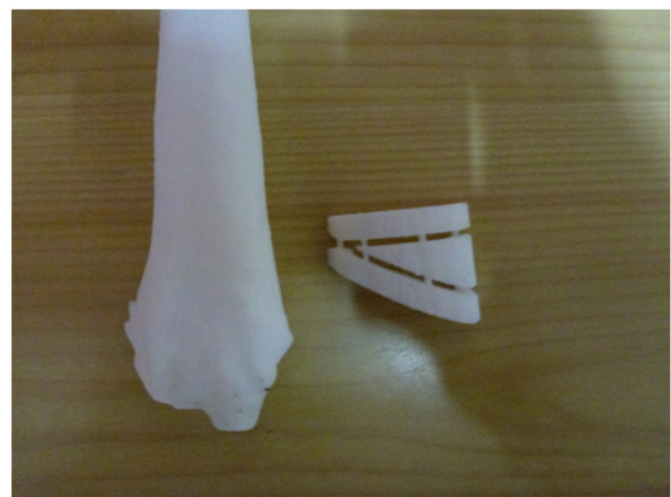
Figure 1F: The guide device manufactured by means of professional rapid prototyping using Acrylonitrile Butadiene Styrene (ABS) material; rehearsal surgery was performed "in vitro" using the guide device in a stereo-lithographic model (F).
