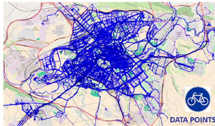
Figure 3: Origin of the one-off measurements of nitrogen oxides (NO x ) carried out at various points in the town of Pamplona by cyclists equipped with connected mobile micro-sensors [29].
