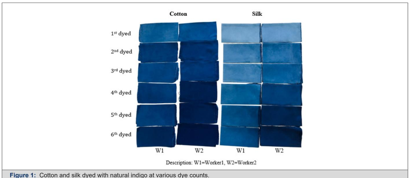
**Figure 1:** Cotton and silk dyed with natural indigo at various dye counts.
