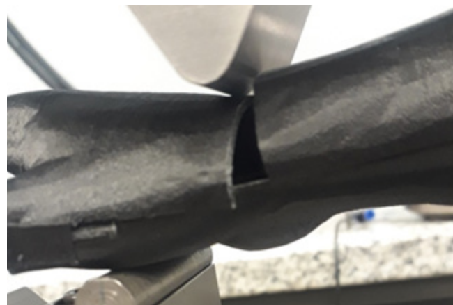
Figure 9: Detail of the failure zone during the flexural test.
