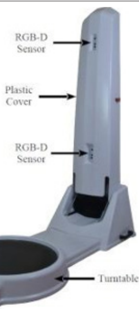
Figure 7: Multifunctional 3D scanner developed at the Federal University of ABC.
