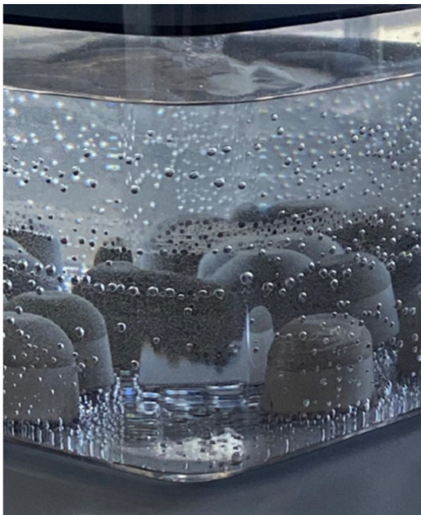
Figure 2: The material that reproduces the dissociation of water, like what happens inside the human eye, is observed at the bottom of the flask. The oxygen bubbles that are constantly released are visible to the naked eye.
