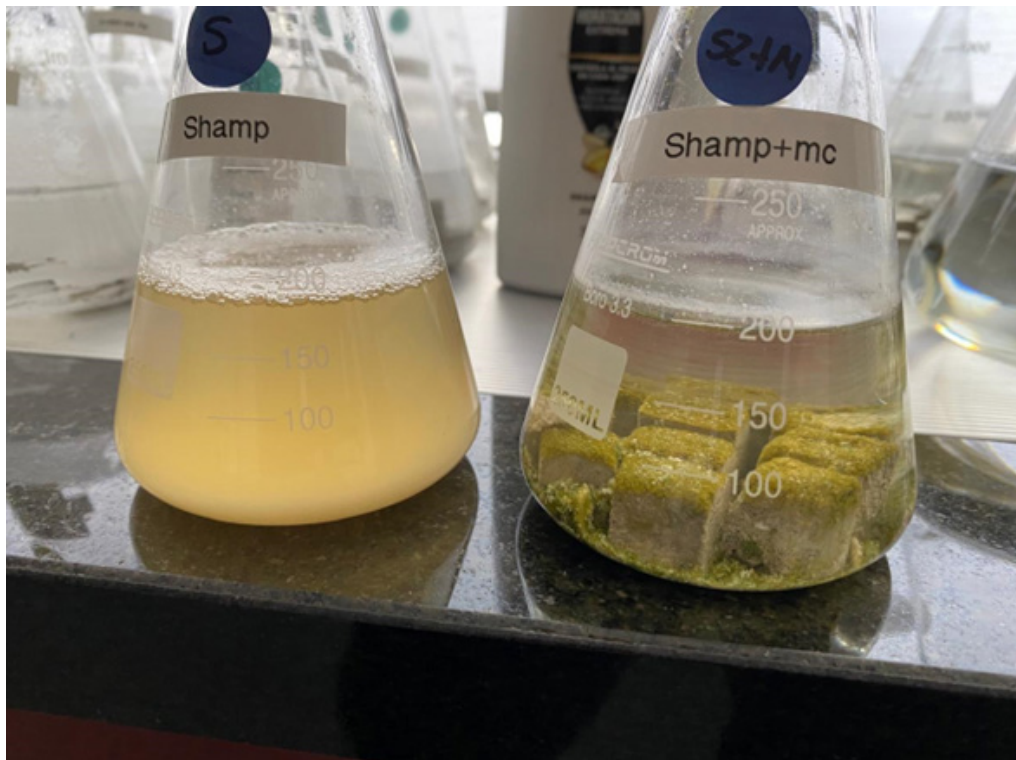
Figure 3: The material developed at the Center for the Study of Human Photosynthesis™, S.C. marketed under the name QBLOCK™, it efficiently clarifies, and without the need for electricity, frequent polluting elements, such as detergents, with little formation of toxic sludge. The quality of the water obtained favors the formation of organic carbon (green zones).
