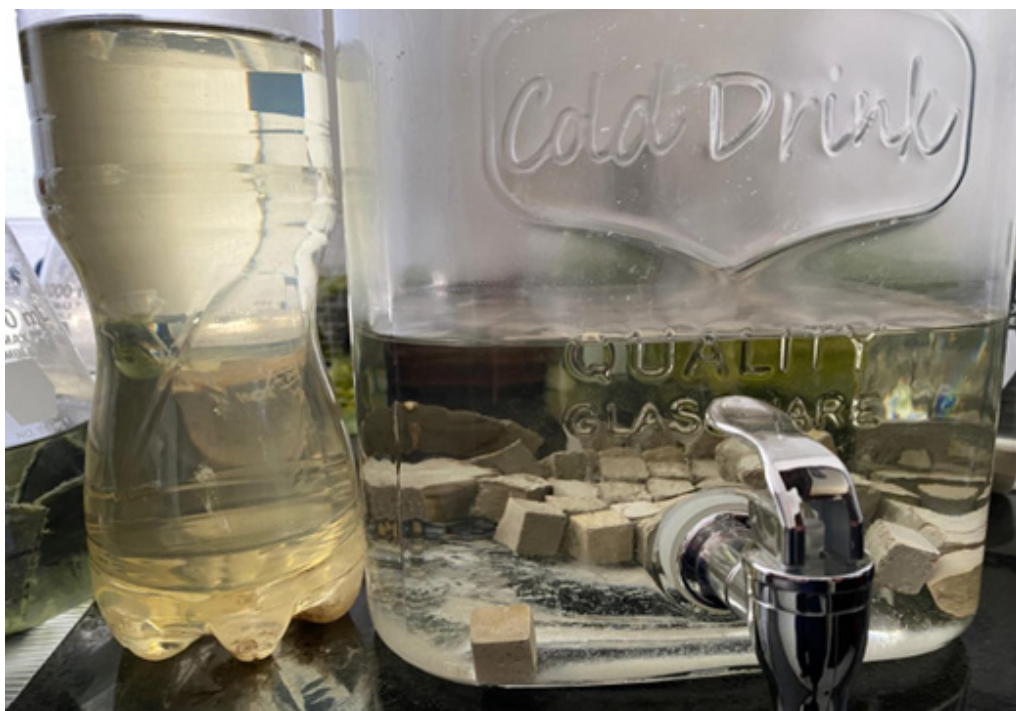
Figure 4: In wastewater containing sugar residues, such as in the manufacture of tequila (right), after 8 weeks, the improvement in the clarity of the water is visible to the naked eye (left), and the low presence of residues at the bottom.
