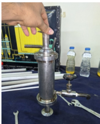
Figure 5: Membrane module made up of SS316.
