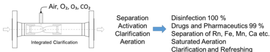
Figure 4: OxTube Machine and its functions in one [5].
