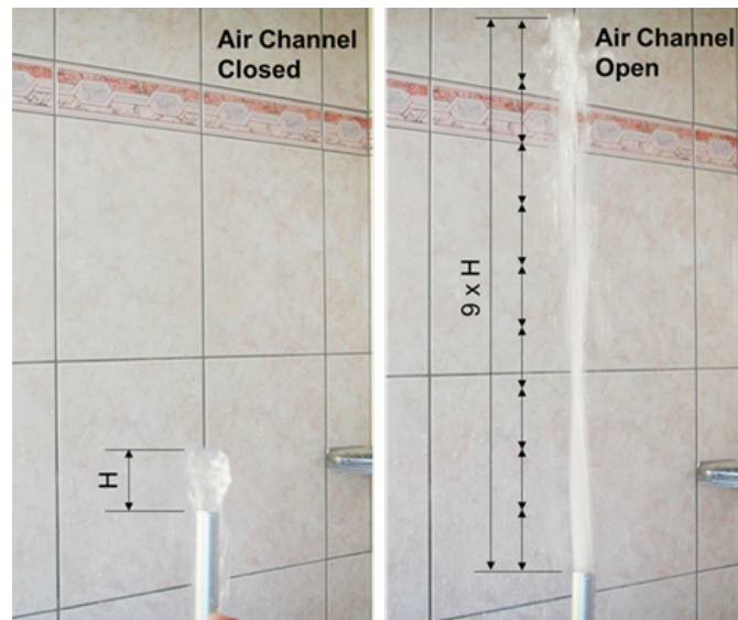
Figure 3: Height of the mixture is nine times higher than the plain water has in the exact same condition of water intake. Air suction could be over 10 times of water in volume at NP [4].
