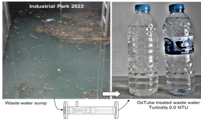
Figure 4: Ox Tube test runs of an industrial wastewater resulted turbidity of 0.0 NTU and zero smell. The clarified water is recyclable in industrial process use [9]. The wastewater is clarified and aerated, and with ozone feed the water is disinfected, too.
