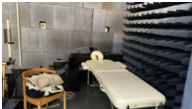
(7.a) Anechoic chamber at IUT Toulouse Blagnac. needles in The pyramidal RF-absorbing foam attenuates ambient electromagnetic interference and the supine bed provides a reproducible subject position across sessions.
